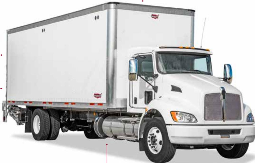
**Seamless, encapsulated foam design** prevents moisture from migrating into the foam and interior. The **smooth sidewall** is perfect for easy cleaning.
