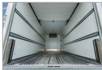
Fork truck rated floor system and sidewalls
