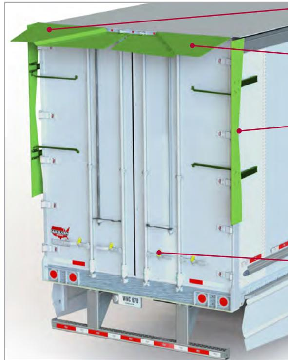
Top panels fold automatically when lock rod is disengaged and door is opened
