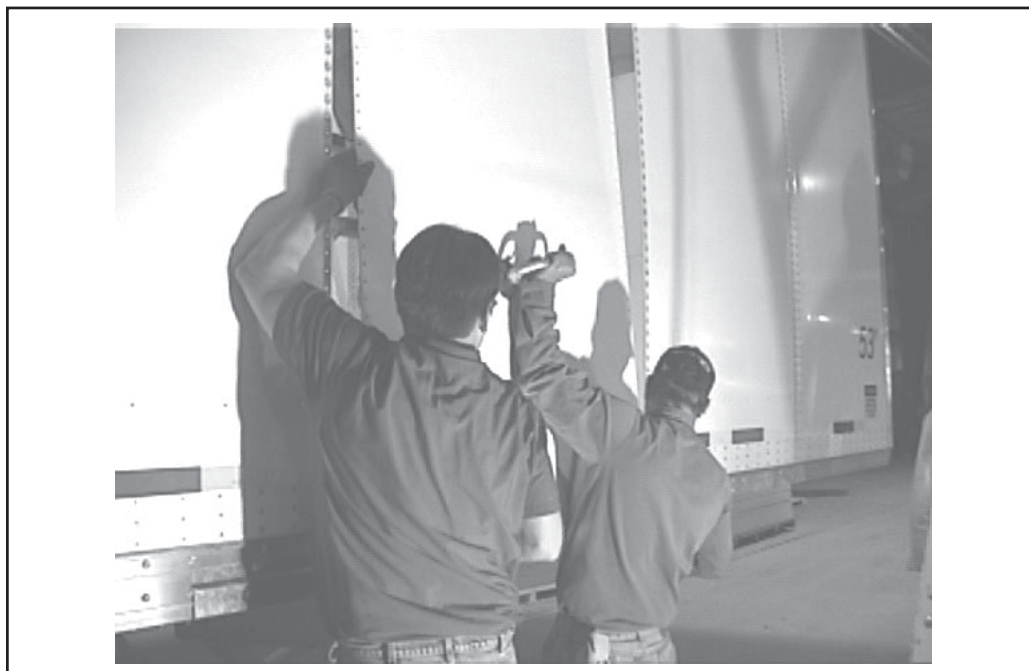
Figure 2-7, Installing the New Panel in the Opening
