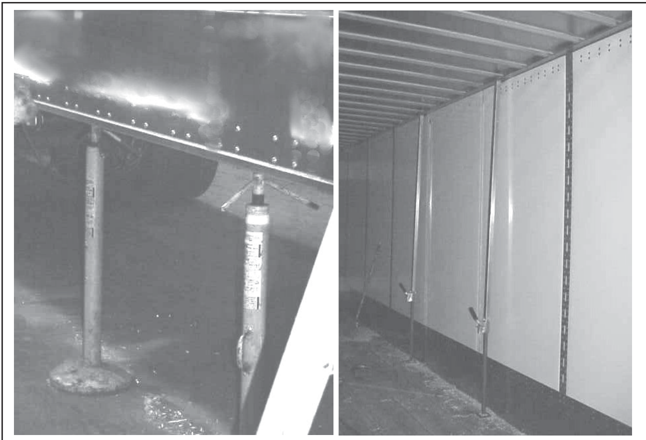
Figure 3-1, Supporting the Base Rail
