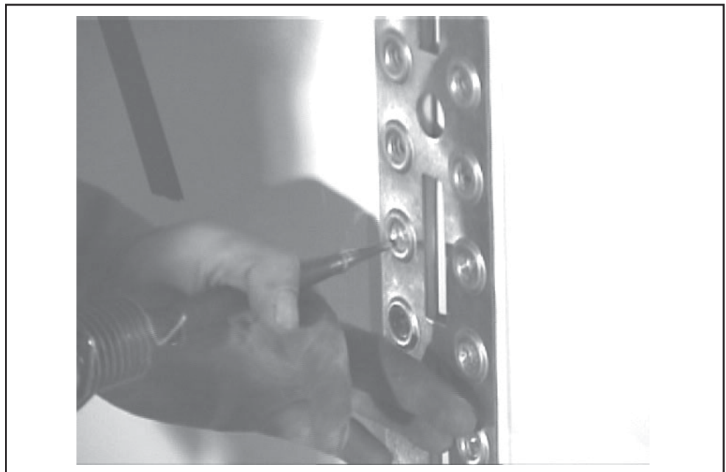
Figure 2-4, Punching Out Rivet Stem Bodies
