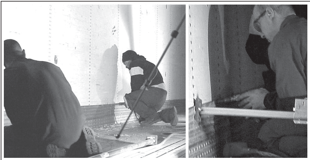
Figure 2-12, Riveting the Scuff Liner to the Side Panel
