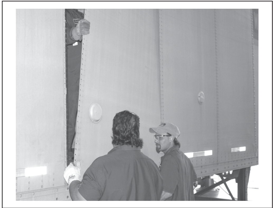
Figure 2-5, Three People to Safely Remove the Old Panel
