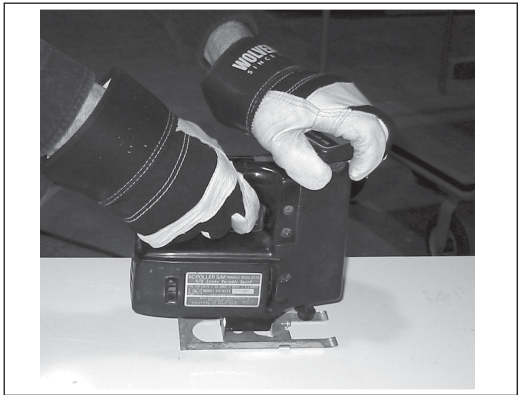
Figure 3-6, Saw Cutting the New Panel to Length—Vertical seam offset must be placed facing the trailer interior to ensure flush surface, preventing freight damage.
