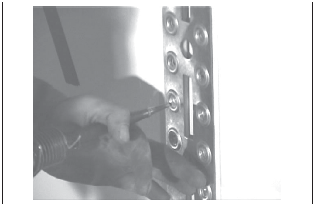
Figure 3-3, Punching Out the Rivet Bodies from Inside
