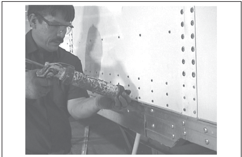
Figure 2-13, Caulking the Base Rail
